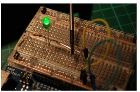
Instead of a push-buttons to close a circuit, it is also possible to use reed switches. Instead of pushing, they react to a magnetic impulse.
