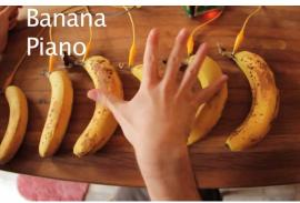
MaKey MaKey is an invention by MIT Media Lab graduates Jay Silver and Eric Rosenbaum. It enables everything, that is at least a tiny bit conductable to turn into a key for your computer. It can detect if a circuit between an object and another object - both connected to the MaKey MaKey using alligator clips - is closed or not.
